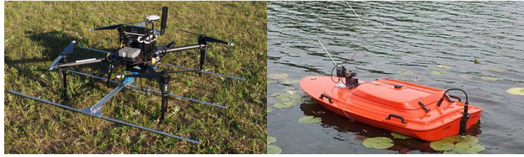
Fig. 1: The target localization problem: given noisy relative measurements, the goal is to localize the targets as quickly as possible using a robot, possibly with complex dynamics such as a quadrotor (left) or surface vehicle [1] (right).
